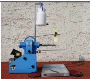
KMK1 the lathe for engraving glass
